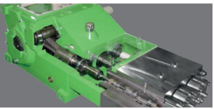
With integrated gear reduction and compact dimensions, KAMAT high-pressure pumps are the ideal tool for numerous applications. Simple operation and maintenance are defining features of KAMAT plunger pumps, as are high modularity and flexibility in regard to delivery rates, pressure settings and fluids. For operating pressures from 0 to 3,500 bar, the input power ranges from 45 to 1200 kW.
