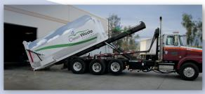
After processing, the odorless, inert waste is safely hauled in the sealed container to a sanitary landfill. Large tonnage loads are possible due to the integrated compactor.
