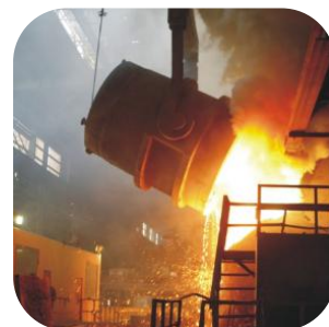
镍铁红送AOD炉 Liquid FeNi charged into AOD
